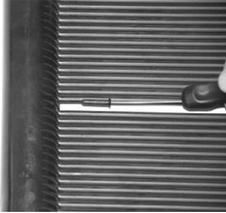
**4.** Gently push the rubber sleeve into the hole created by the removal of the riser, until only the head is showing.
