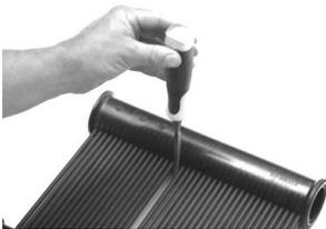
2. Using a  $\frac{1}{4}$  inch chisel, and holding the flat side of the chisel towards the header, cut through the damaged riser, as close as possible to the header. A round hole is created in the manifold header.
