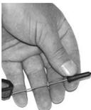
3. Spray the rubber sleeve with lubricant and pull it over a  $\frac{5}{64}$ " Allen Key.
