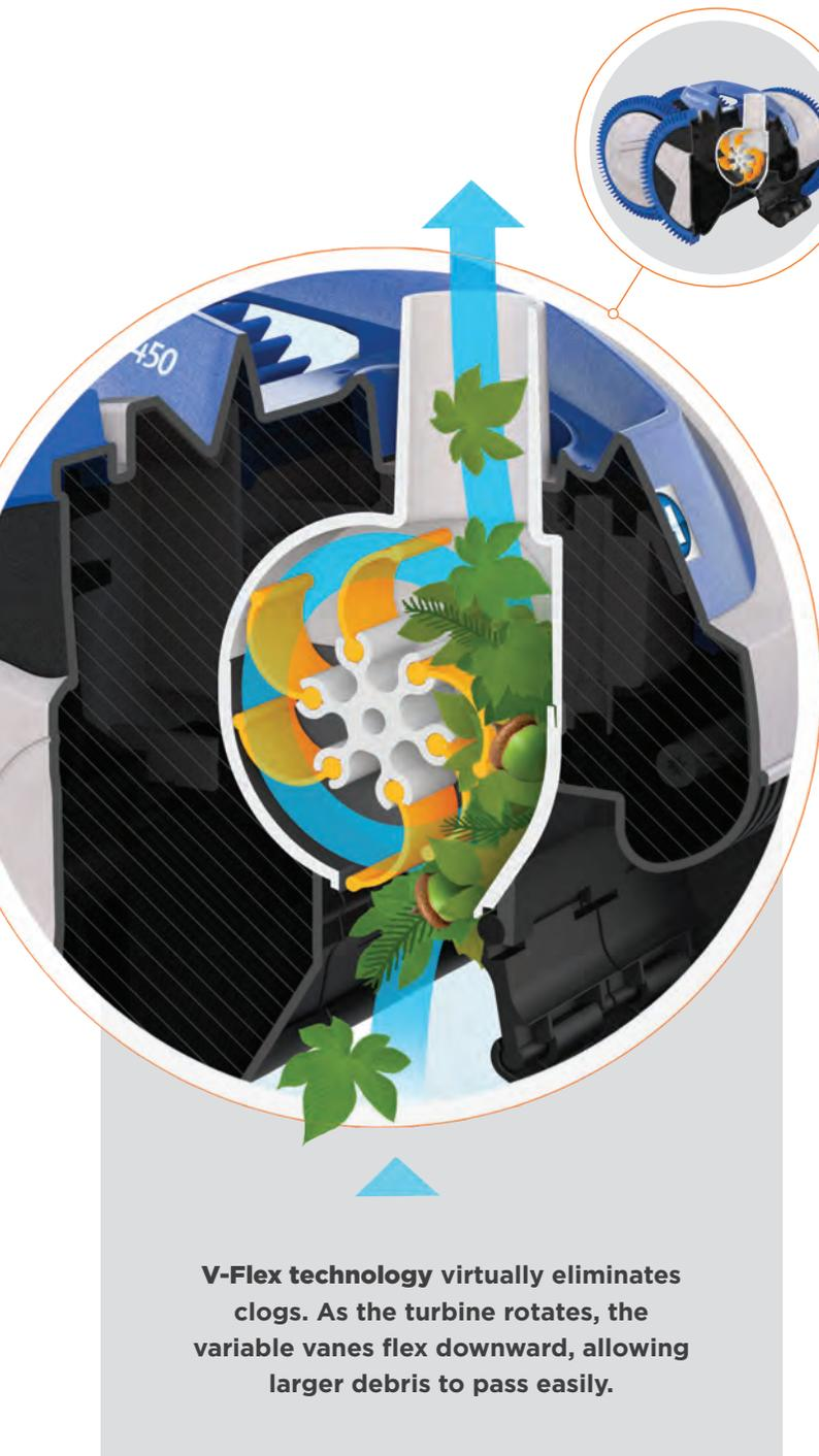
**V-Flex technology virtually eliminates clogs. As the turbine rotates, the variable vanes flex downward, allowing larger debris to pass easily.**
