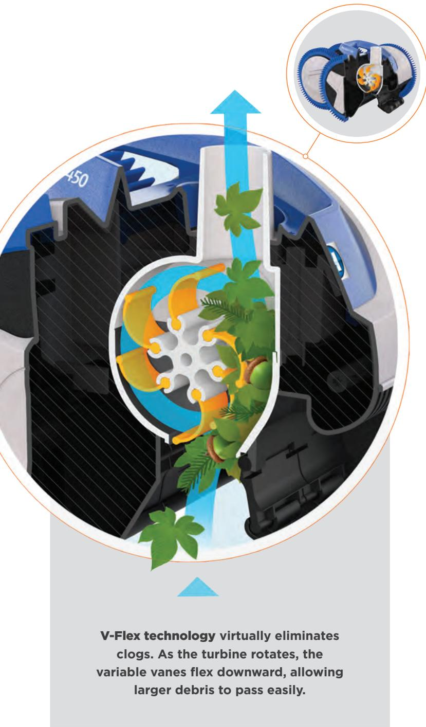
**V-Flex technology virtually eliminates clogs. As the turbine rotates, the variable vanes flex downward, allowing larger debris to pass easily.**
