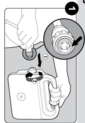
Attach the floating cable to the power supply.
