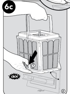
Open the latch to release the bottom lid in order to remove the debris.
