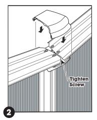
**Important**: When installing the top connector, ensure the front lip of the connector is over the top lip of the bottom connector.
