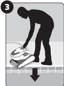
Put the Pool Cleaner into the pool. Release the Pool Cleaner and let it sink to the floor of the pool. Make sure that the floating cable is free of any obstructions.
