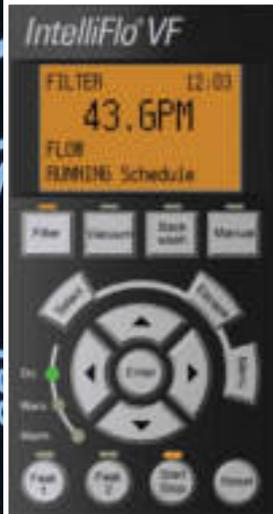
The IntelliFlo VF is the first pump to use a permanent magnet synchronous motor (PMSM). But the real secret is IntelliFlo's powerful microprocessor that senses impeller load, and adjusts motor speed by controlling current frequency and voltage. That's how IntelliFlo is always able to maintain the most efficient flow possible.
