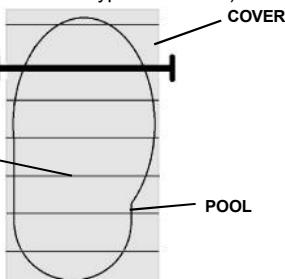
When cutting the cover, allow a 1 1/2" wide border around the pool edge to compensate for shrinkage.
