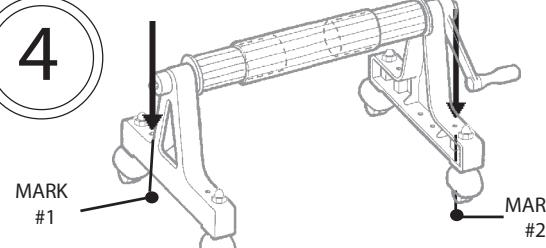
Using one of the two holes in the A-frame as a guide, make mark #1 on deck. With a 1/2" concrete drill bit, drill a 1 1/2" deep hole at mark #1. Complete steps 5 and 6 before continuing with step 4.
