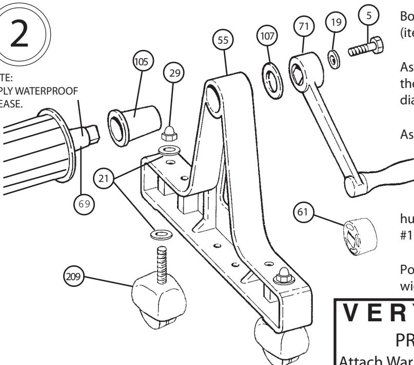
Bolt the castors (item #209) to the A-frames (item #55), as shown in the diagram.
