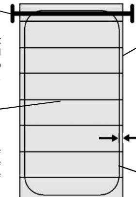
Open cover over the pool and set into position. Ensure that the end of the cover (where it attaches to the roller) is square to the roller.
