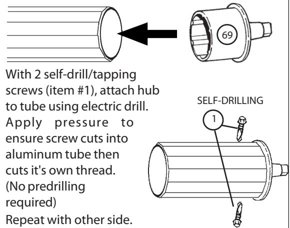
With 2 self-drill/tapping screws (item #1), attach hub to tube using electric drill.
