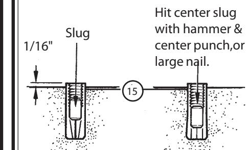
Hit center slug with hammer & center punch, or large nail.
