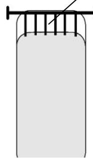
Attach the cut cover to the roller with the blue straps (See grommet detail). Ensure length of strap allows cover to lay flat on pool, to prevent wind from getting under cover.
