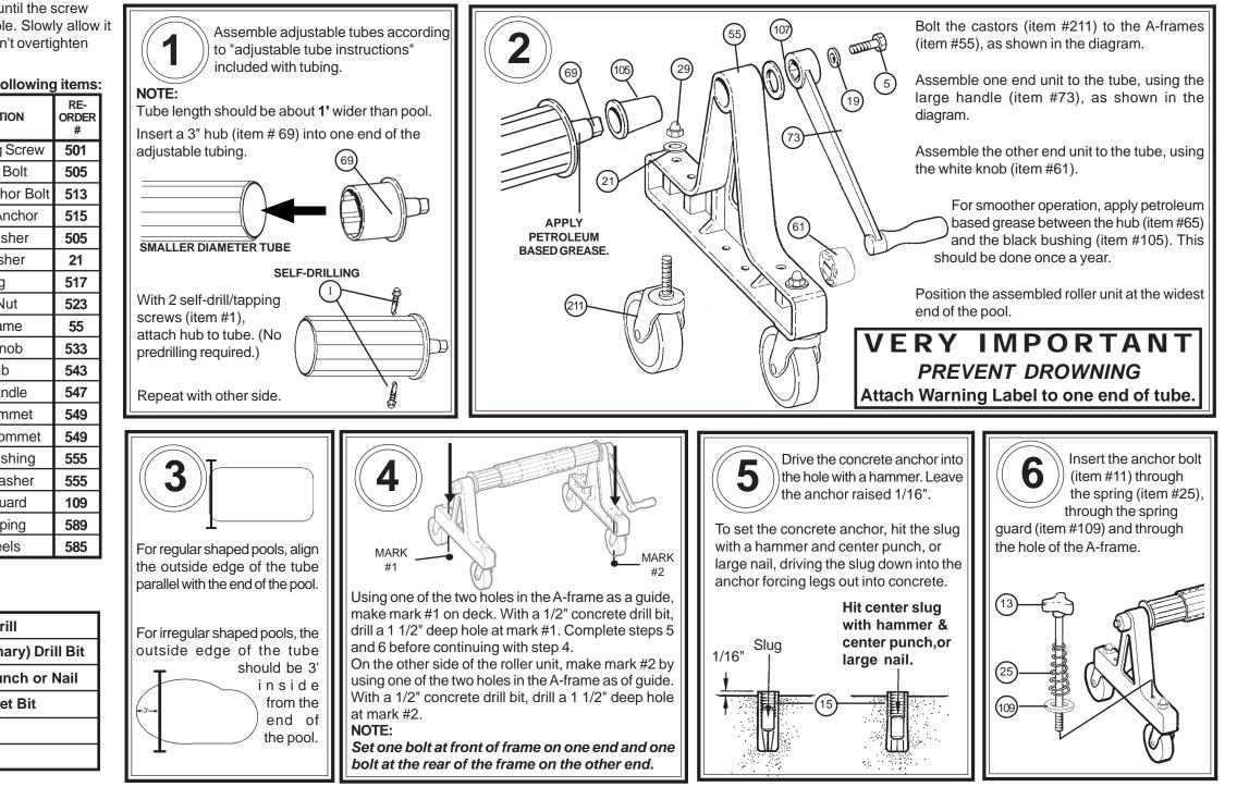
**NOTE:** Self Drilling Self Tapping screws require that you use an electric drill. Apply pressure to drill until the screw starts to cut it's own hole. Slowly allow it to cut screw thread. Don't overtighten screw.
