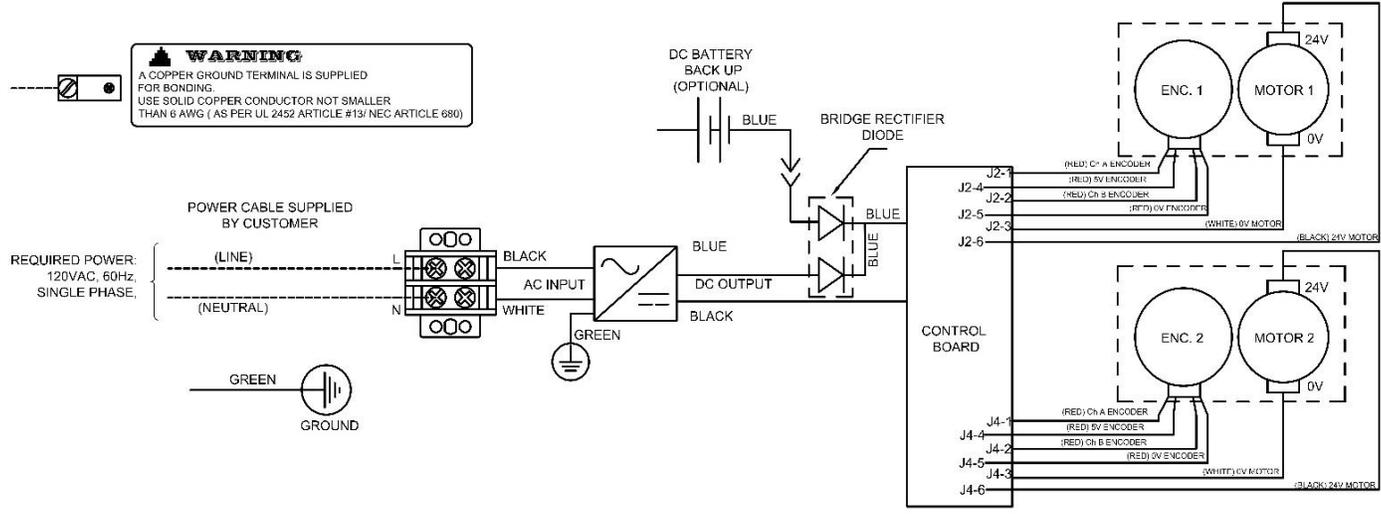
The control circuit operates at 120VAC, 60Hz. Due to the resistance in the wire used to carry the control circuit voltage, it is important to use the appropriate wire size between the AC control box and the main power supply. If wire gage is not suitable for the distance, problems in AC control box will be encountered such as motor humming, premature wear of the power supply and possible tripping of it's thermal protection.
