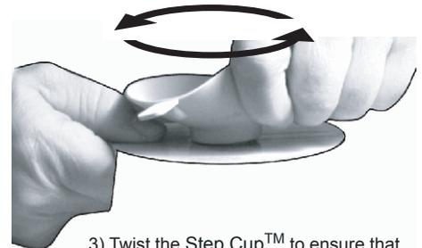
3) Twist the Step Cup™ to ensure that its mushroom has entirely cleared the wall thickness. If it has, the suction cup should rotate freely.
