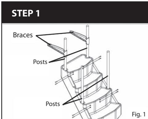
1. Insert the posts into the step and align with the predrilled holes. Attach using the 3" bolts (8), washers (16), and nuts (8). Slide the braces over the posts and leave unattached (Fig. 1)
