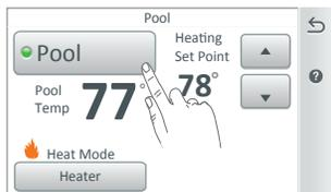
**Pool Filter Pump On/Off:** Tap this button to switch the pool filter pump on or off and to activate the heater (if a heater source is selected).
