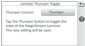
**Gears Icon:** Tap the Gears icon to access the **MagicStream laminar Thumper** feature. Tap the Thumper button to activate the built-in light solenoid to create a random wrinkle in the laminar's water stream and display a brilliant spot of light that moves along the stream's arc.
