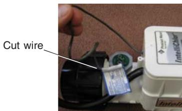
4. Using a flat 1-3/16" (30 mm) wrench carefully unscrew the flow-temperature switch assembly until the switch can be removed from the cell. Be careful not to damage the cell plastic coupling with the edge of the wrench.
