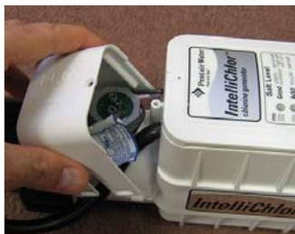
3. Cut the cable close to the switch to allow enough wire for the new switch cable to be connected to.
