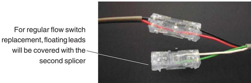
8. Wrap the excess wire around the flow switch.
