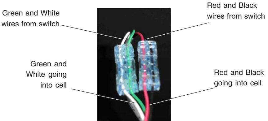
7. If replacing a regular flow switch (RED and BLACK wires only), insert green and white wires from new flow-temperature switch into one end of the second water-tight connector and crimp using pliers. This will provide electrical insulation for the floating leads.
