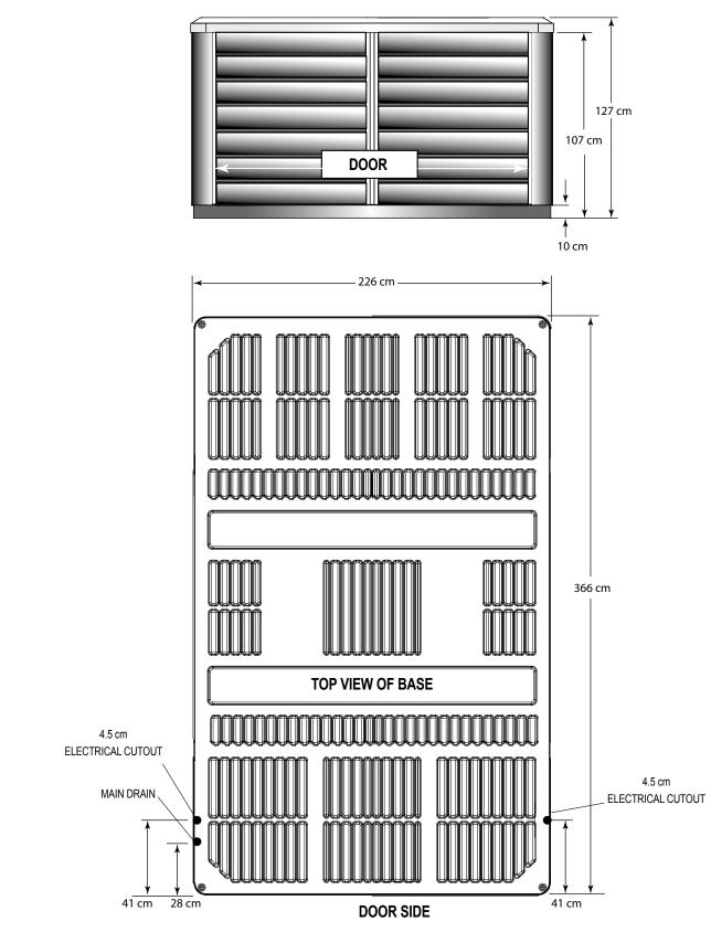
NOTE: ENDLESS POOLS requires that the X200 Model be installed on a minimum 15 cm thick reinforced concrete pad or structurally sound deck able to support the "dead weight" found in the specification chart on the back page.
