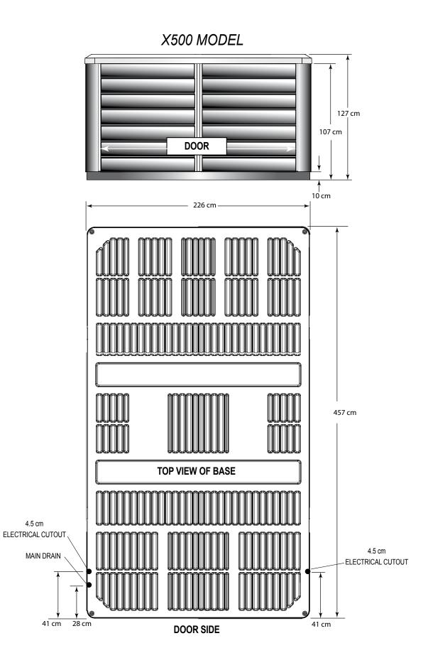
NOTE: ENDLESS POOLS requires that the X500 Model be installed on a minimum 15 cm thick reinforced concrete pad or structurally sound deck able to support the "dead weight" found in the specification chart on the back page.
