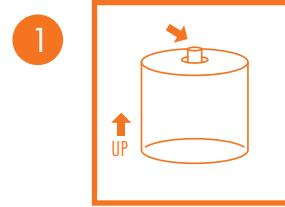
Make sure Luci is facing upward (valve on top, battery on bottom)
