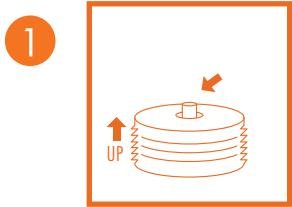
Make sure Luci is facing upward, (valve on top, battery on bottom)
