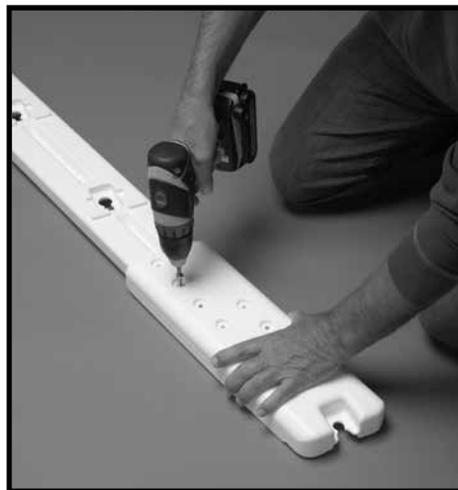
**#2:** Using two 1/4-20 x 1 1/2” long bolts and two 1/4-20 hex nuts, fasten the Adjustable Rail Boot to the Side Rail. Repeat for remaining three Side Rails.
