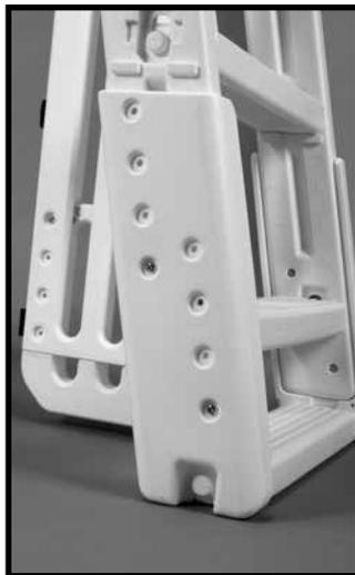
**#3:** Check to make sure the hole locations in the platform are clear of pool wall and supports. Drill two 5/16" holes through the Platform and pool ledge. Fasten the ladder platform to the pool ledge using two 1/4-20 x 2-1/4" bolts, 1/4-20 hex nuts. **You MUST secure the ladder to the pool top rail for strength and stability.**
