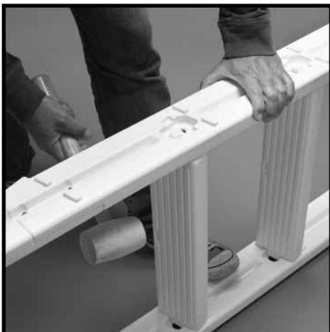
**#4:** Place the opposite Side Rail assembly on top of the Fixed Ladder Treads so that the notches and tabs align and tap it into place. Placing your foot on the Side Rail to hold it steady, use the rubber mallet to tap down the Fixed Ladder Treads until they are firmly seated into both Side Rails.
