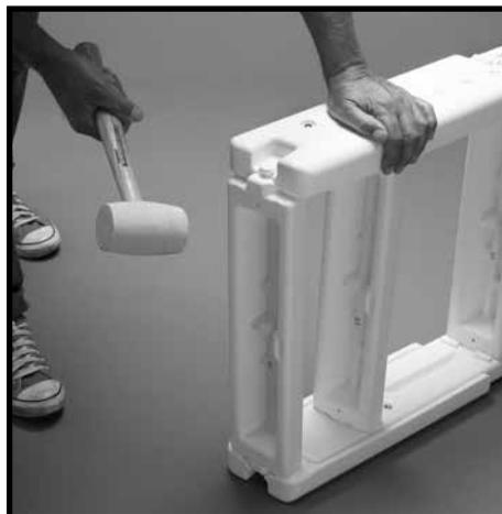
**#5:** With ladder assembly on edge, position one of the remaining Fixed Ladder Treads so that the tabs align with the notches at the bottom of the Side Rail assemblies and tap in with the rubber mallet until the tread is properly seated.
