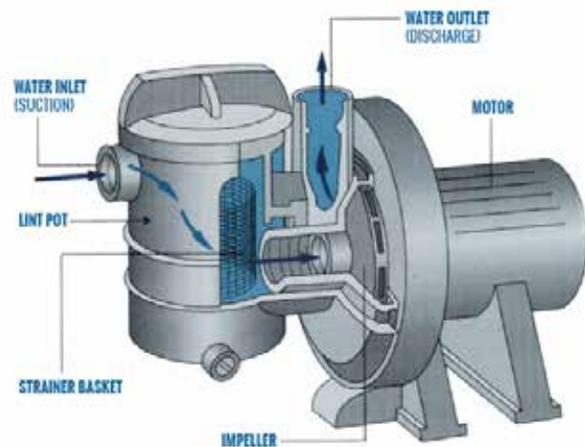
A pump and motor is used to draw water from the pool. The pump is generally the only active or powered component of your pool equipment. In essence, it is the 'heart' of your system, drawing the water from an opening in the pool wall called the skimmer, and then directing it under pressure to the filter tank where it is cleaned and returned to the pool. When the pump is off no other equipment can operate.
