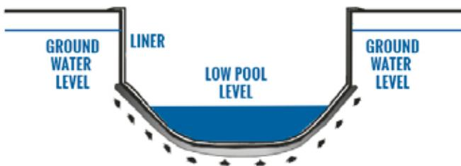
If the pool water level is low and if ground water is high as in the following illustration the water in the ground wants to make the pool and its' liner float.
